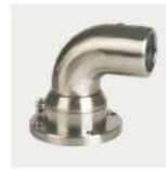
Pipe Connector Order Nr. 4820 Weight: 3.5kg Material: stainless steel Rotatable angle: 0-320°
