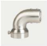
90° Box Connector Order Nr. 4850 Weight: 2.3kg Material: stainless steel Rotatable angle: 0-320°
