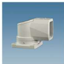
Top Base Order Nr. 440.6.120.00 Weight: 1.13kg Material: die casting aluminum alloy Horizontal Rotation Angle: 0-320°
