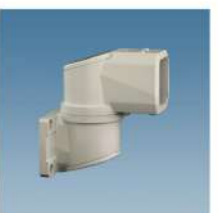
Horizontal Wall Base Order Nr. 440.6.110.00 Weight: 1.36kg Material: die casting aluminum alloy Horizontal rotation angle: 0-320°
