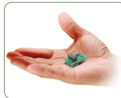
As the world's smallest serial-to-Ethernet module, the thumb-sized MiiNePort maximizes your design flexibility.
