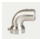
90° Box Connector Order Nr. 4850 Weight: 2.3kg Material: stainless steel Rotatable angle: 0-320°
